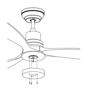
Attach the lamp panel with the three screws on the fan.
