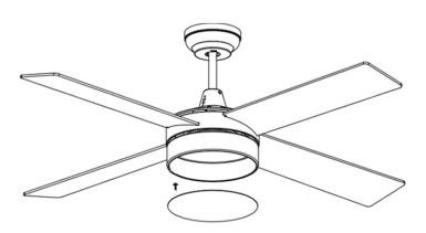
Push the cover diagonally into the lamp panel
