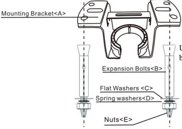
Use a power drill and anchor to drill the mounting bracket into the concrete ceiling.
