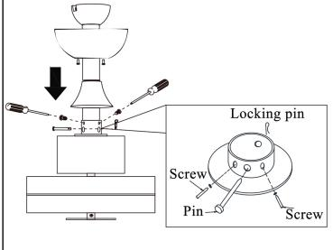
Assemble the ceiling fan. Attach the downrod to the flange on the top the motor with screws, bolts and pins.
